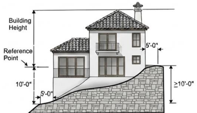
Figure 16.18-5 - Stepped Building = \geq 10'-0"
