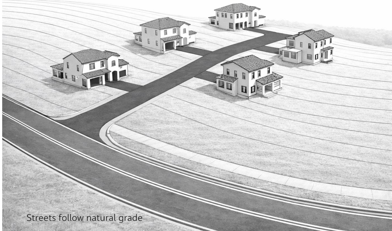
FIGURE 16.24-12 ROADWAY PLACEMENT AT A SITE
