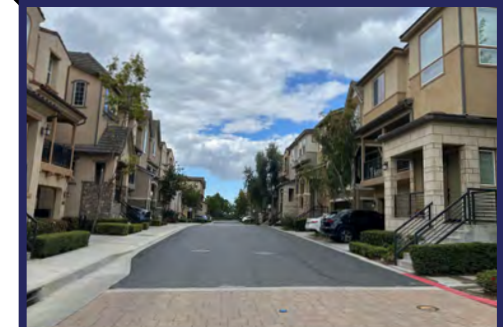
Residential lanes provide vehicular and pedestrian access to multiple residences in the form of a shared street. This street type features distinct entry paving and landscaping to demarcate the lane's dual functions.
