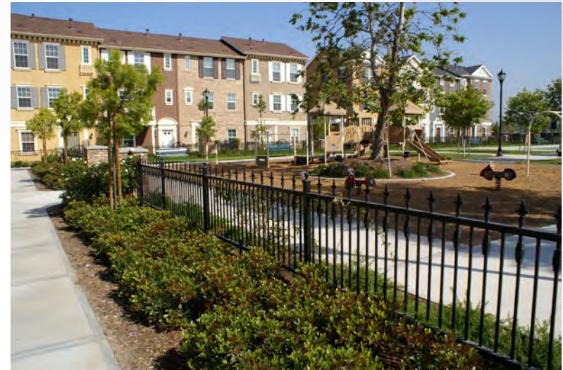
Children's play areas shall be protected from any adjacent streets or parking lots with a fence or other barrier at least 4 feet in height.
