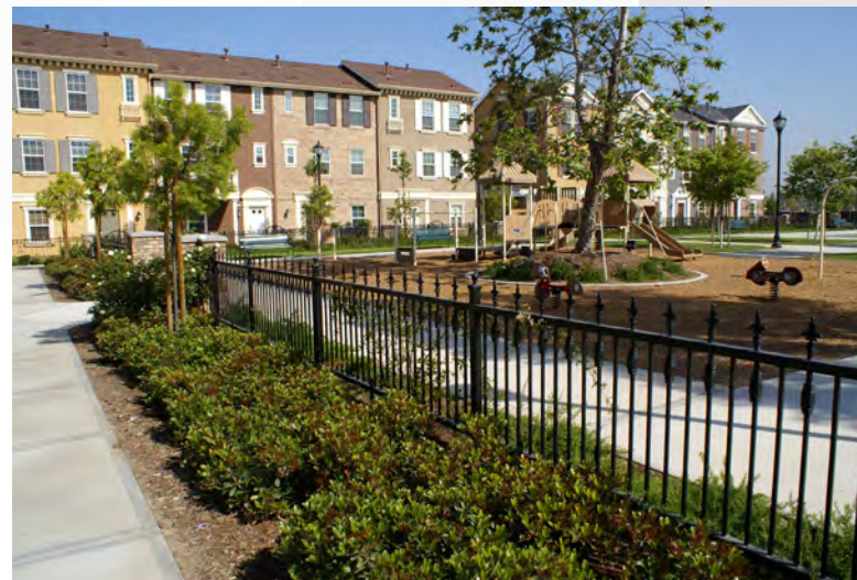
Children play area shall be protected from any adjacent streets or parking lots with a fence or other barrier at least 4 feet in height.
