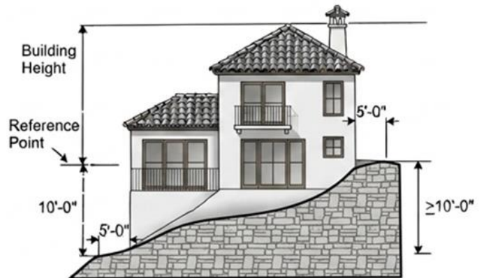
Figure 16.18-5 - Stepped Building = \geq 10'-0"
