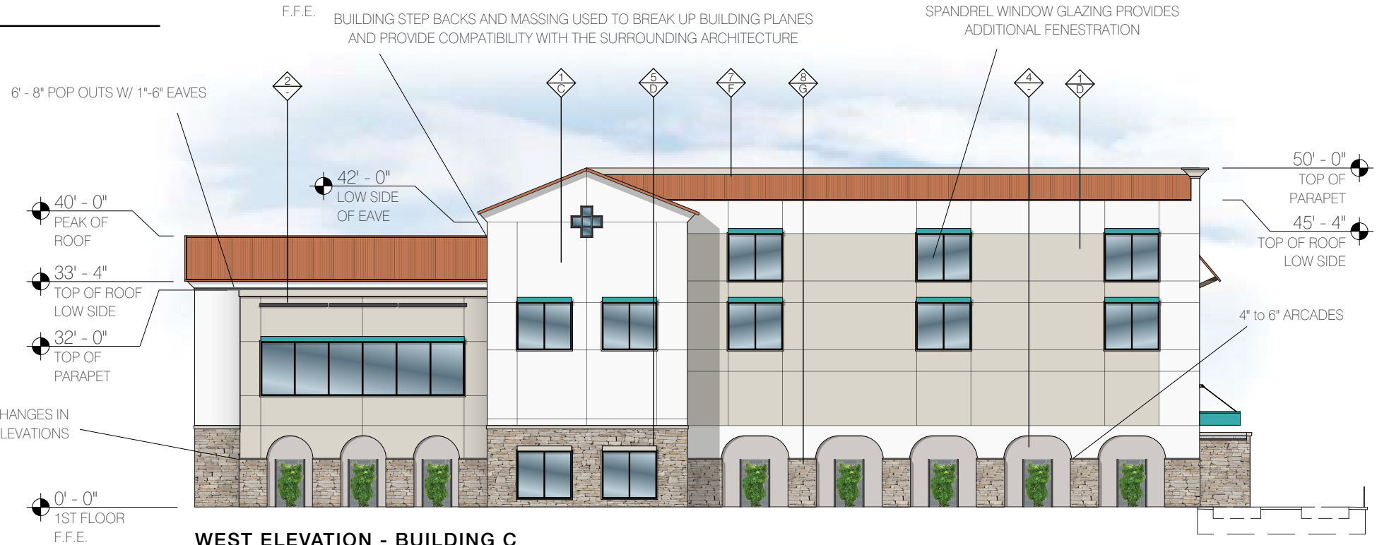
WEST ELEVATION - BUILDING C Scale: 1" = 20'
