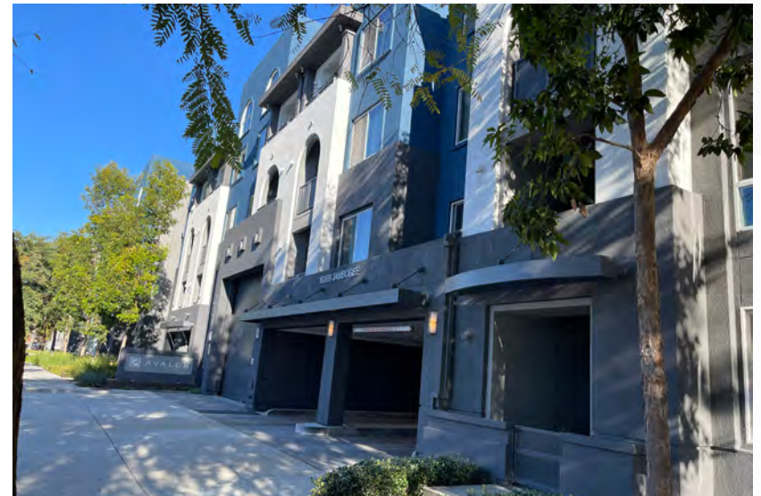
Any driveway providing access to a parking structure shall have a minimum width of 28 feet.
